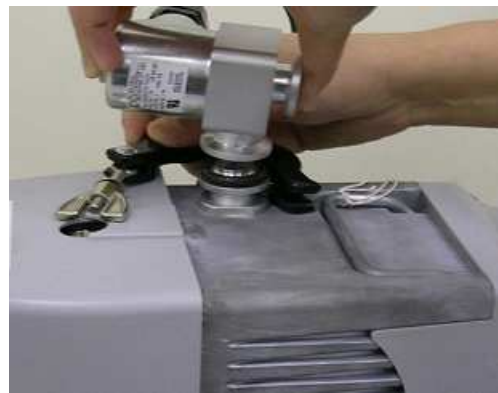
Figure 9 Mount Inlet Valve with IDP-3 Pump
