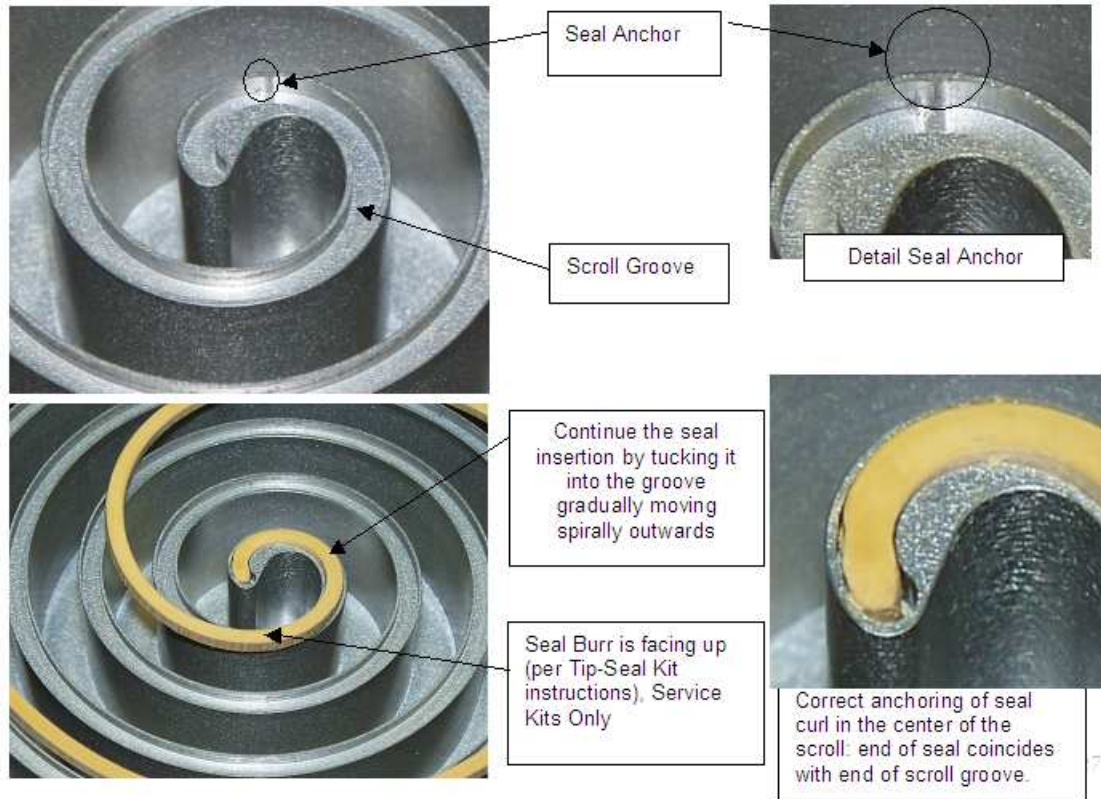
Figure 11 Tip Seal Seating
