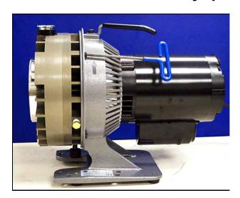
6. Secure pump module to frame with four M6x16 screws.
