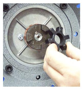
4. Insert spider in motor coupling.
