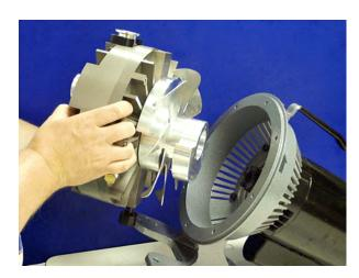
4. Remove pump module from the frame.
