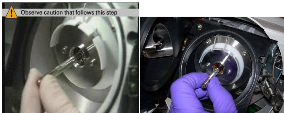
Figure 45 Pulling the capillary out of the desolvation assembly
