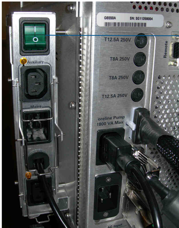
Figure 8 Power connections and pump expander box behind service panel for 6400 Series and 6500 Series instruments with a pump expander box,
