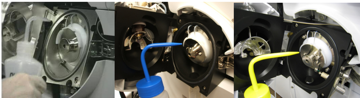
Figure 24 Rinsing the area around the spray shield for 6100 Series (left), 6200 Series (center) and 6400/6500 Series LC/MS
