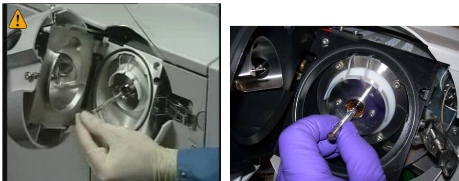
Figure 46 Reinstalling the capillary
