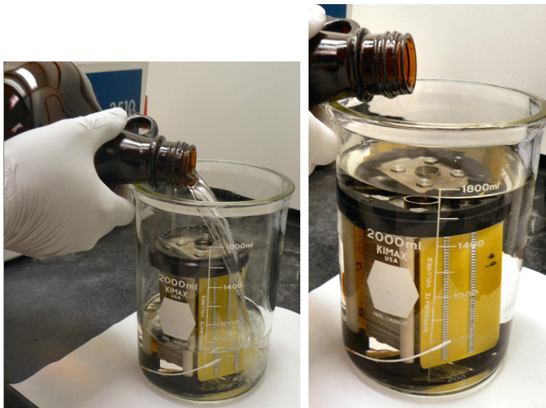
Figure 51 Pouring isopropanol into the glass beaker.
