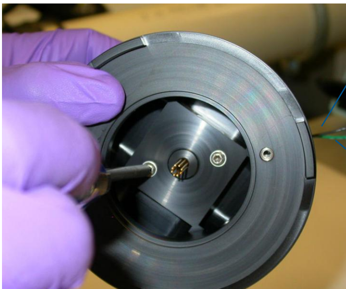
Figure 65 Remove these two 8-mm T10 Torx screws to remove the skimmer for better access to the rods for cleaning.
