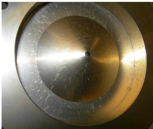
Figure 56 Sample residue on skimmer
