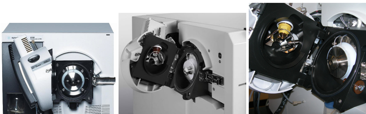
Figure 20 Opened AJS spray chamber for 6100 Series (left), 6400 Series (center) and 6500 Series (right) LC/MS.
