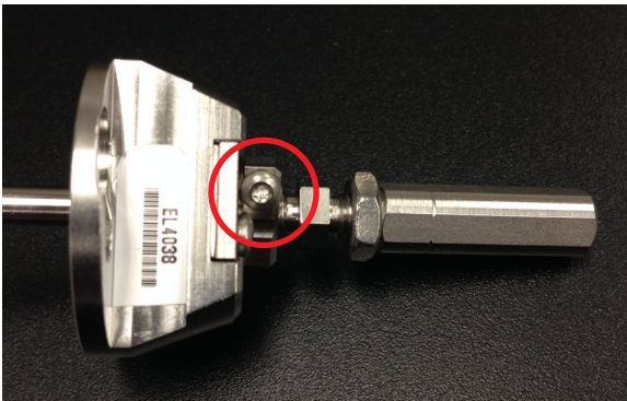
Nebulizer with T6 Torx screw (screw p/n 0515-0677)
