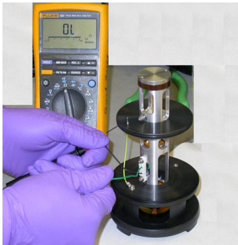
Figure 67 Testing for continuity.
