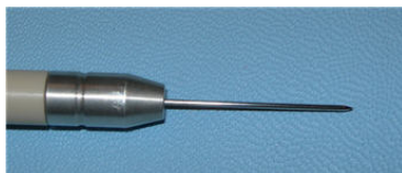
Figure 36 APCI corona needle after cleaning.
