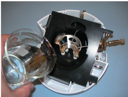
Figure 21 Filling the ESI spray chamber for 6100/6400 Series (left) and 6200/6500 Series LC/MS
