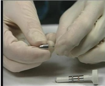
Figure 38 Installing a new needle into the collar
