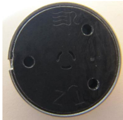
Figure 17 CDS rotor seal in its proper orientation
