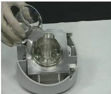
Figure 21 Filling the ESI spray chamber for 6100/6400 Series (left) and 6200/6500 Series LC/MS
