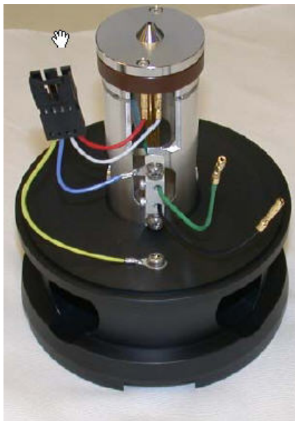
Figure 80 The re-assembled ion optics assembly
