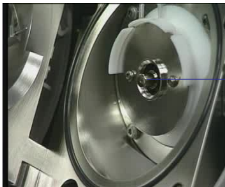
Figure 16 End of capillary cap
