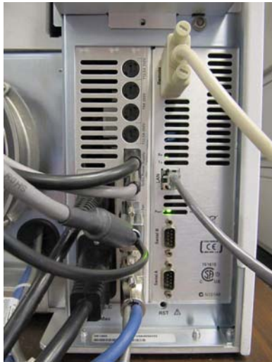
Figure 66 Disconnect the instrument power cable.
