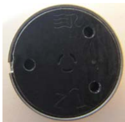
Figure 48 CDS rotor valve in its proper orientation
