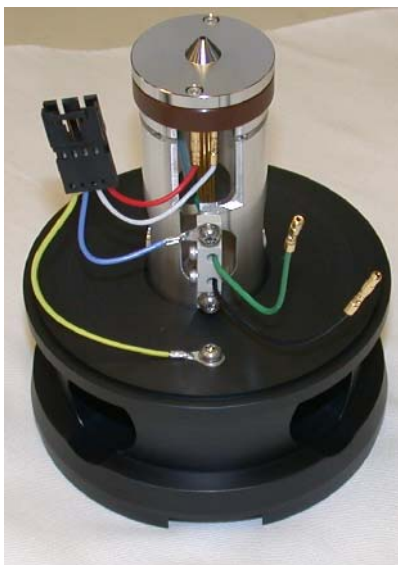
Figure 52 Ion optics assembly
