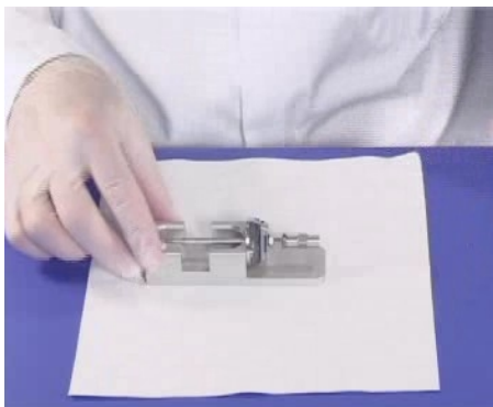
Figure 6 Electrospray nebulizer needle in needle holder
