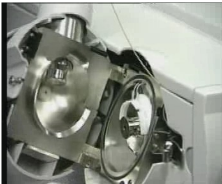
Figure 27 Opened spray chamber
