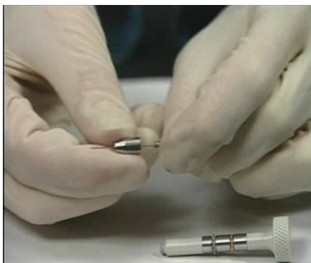
Figure 35 Installing a new needle into the collar
