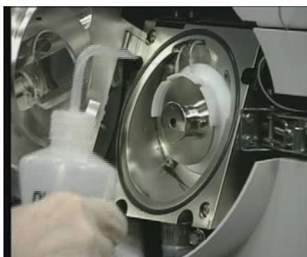
Figure 17 Rinsing the area around the spray shield
