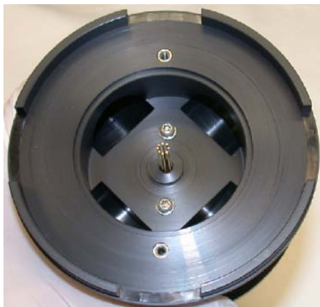
Figure 54 Octopole rods extending through Skimmer Spacer.
