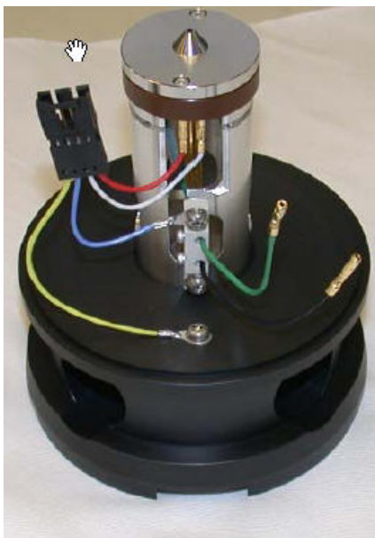
Figure 62 The re-assembled ion optics assembly
