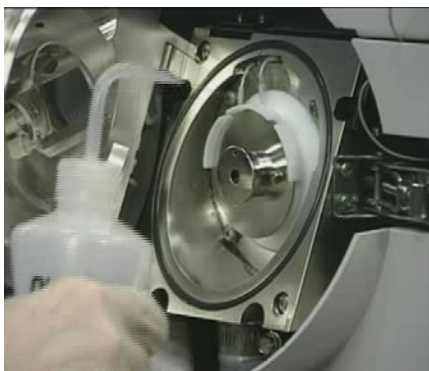
Figure 4 Rinsing the area around the spray shield
