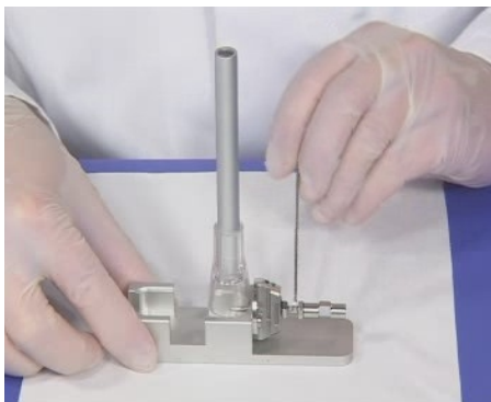
Figure 32 Installing the nebulizer in the adjustment fixture
