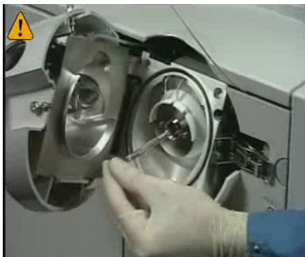
Figure 38 Reinstalling the capillary
