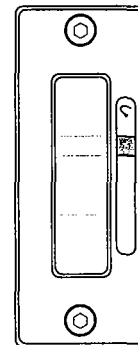
Oil level sight glass for "SD" series pumps except 1015 SD, 1021 SD
