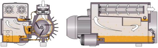
The vacuum pump works on the rotary vane principle.
