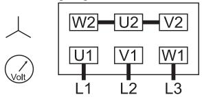
Double star connection, multi-voltage motor (low voltage):
