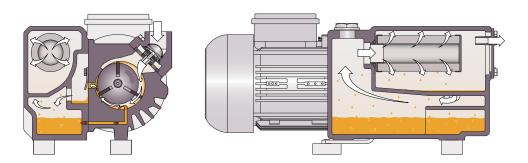
The machine works on the rotary vane principle.
