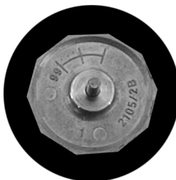
Figure 15 - Position a new diaphragm
