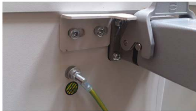
Figure 12 - Protective Earth (PE) connection
