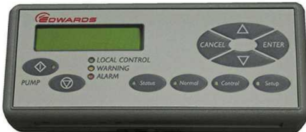
Figure 19 Pump display terminal
