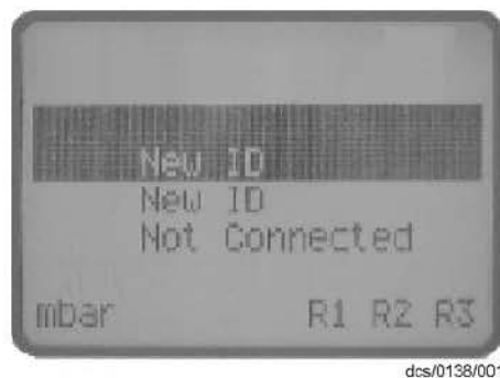
Figure 16 - New gauge connected
