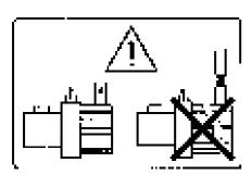
Warning - do not block the pump outlet.
