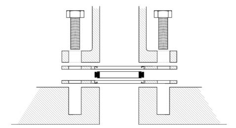
Figure 5 - Connect inlet to NW40 inlet fittings
