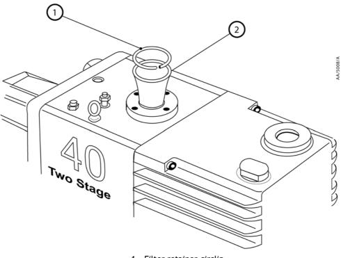
Figure 7 - Remove and replace inlet-filter
