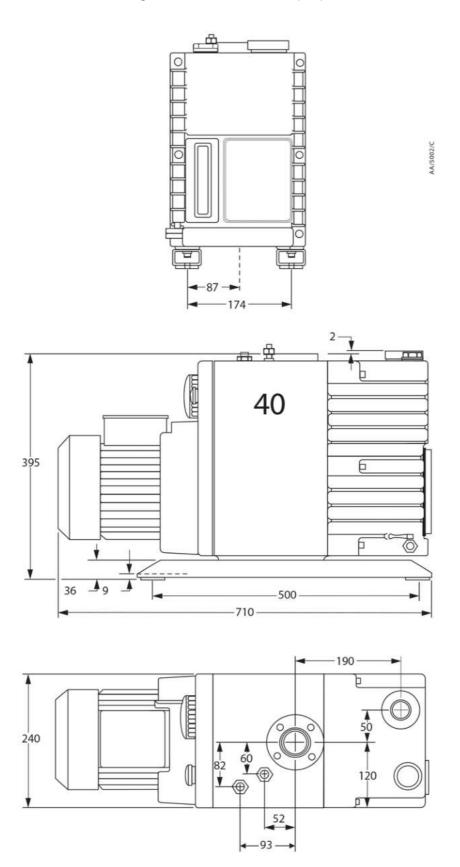
Figure 3 - Dimensions E2M80 (mm)
