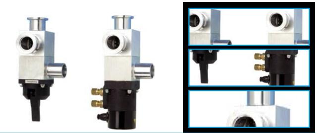
Edwards backing/roughing valves with ISO NW roughing and forepump terminations feature manual or pneumatic actuation. They combine the function of separate backing/roughing valves in one integral 3 port unit.
