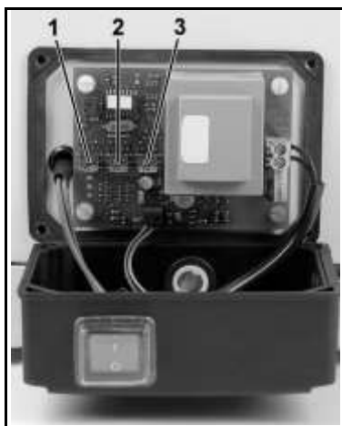
Fig. 5: Control box (opened) of drying system with switches 1, 2, 3
