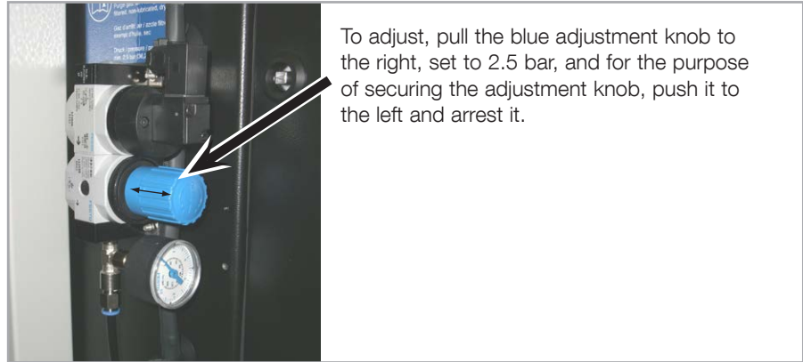
Fig. 4.5 Adjust the pressure reducer
