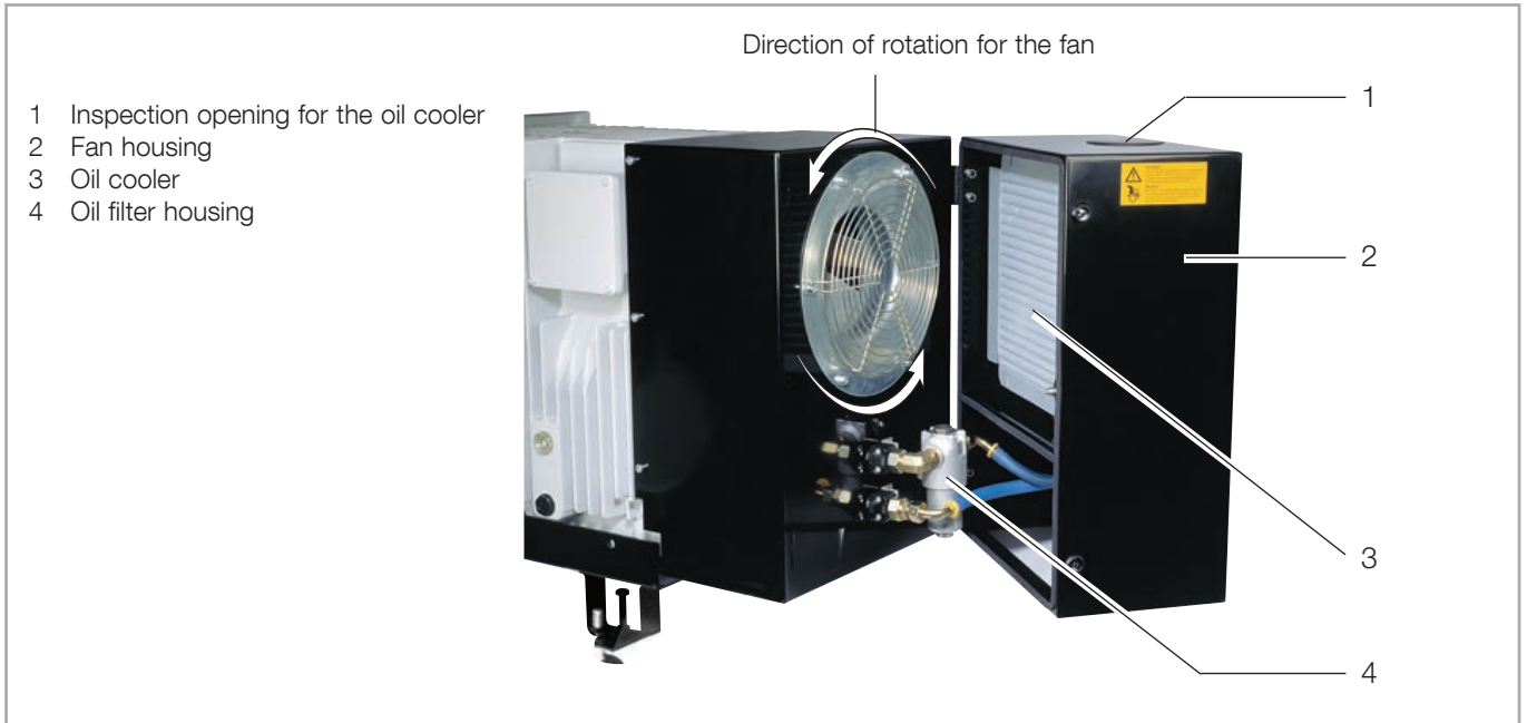
Fig. 5.1 Opened fan housing
