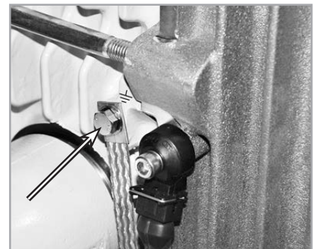
Fig. 3.6 Ground connection example
