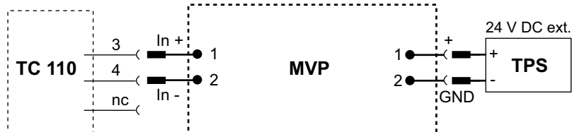
Fig. 5: Connection to TC and TPS
