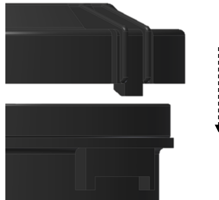
Figure C.5.2: Canister securing position for housing without elements.
