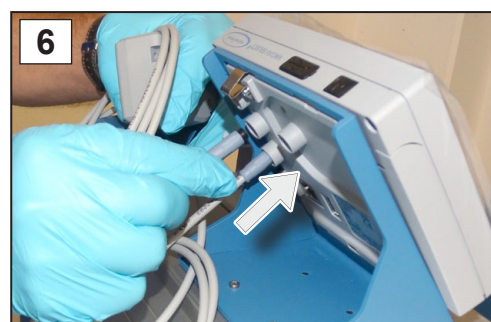
6. Also plug in the VACUU·BUS cables from peripheral devices. Use Y adapters (accessories) if there are not enough connections.
