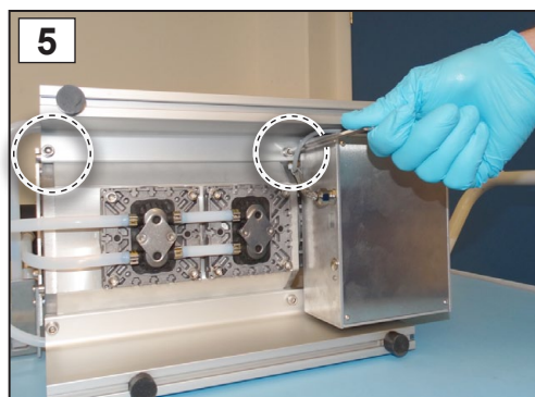
5. Wind the screw fittings into the side panel; hex key size 5.
