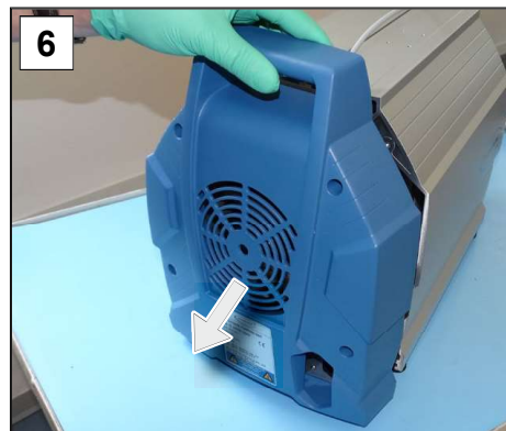
6. Remove the housing section and set it aside.
