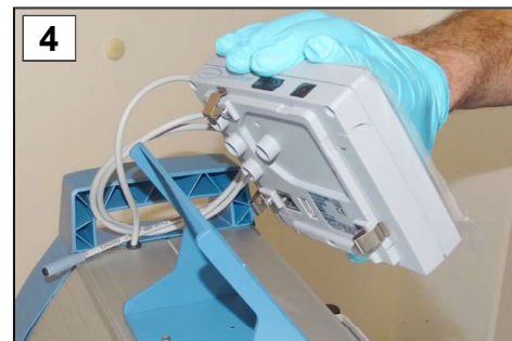
4. Clip the controller into the base.
