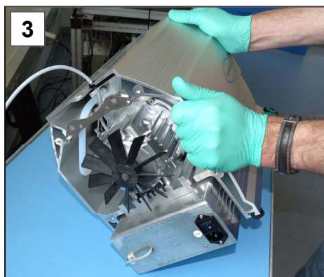
3. Place the pump carefully on its side.
