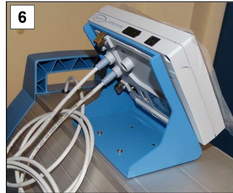
6. Secure the controller on the diaphragm pump and connect all cables.
