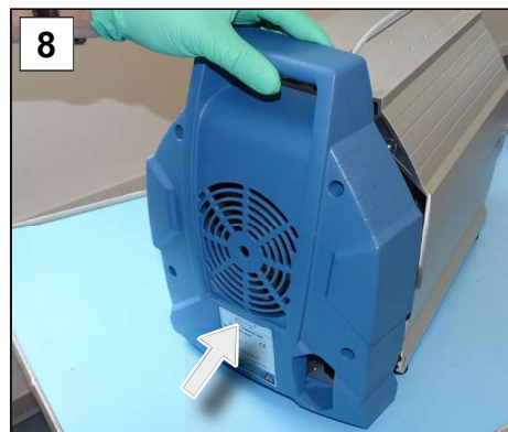
8. Place the rear housing section.
