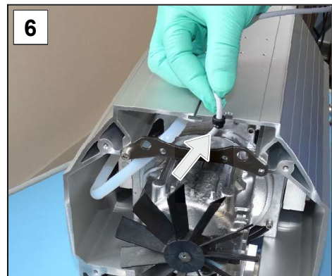
6. Secure the cable in the rear recess.
