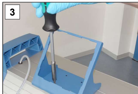
3. Screw the base onto the diaphragm pump.
