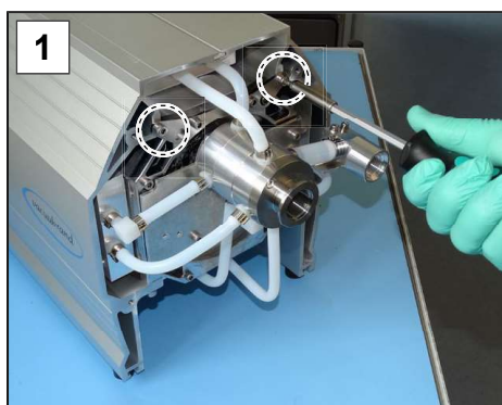
1. Unscrew the 2 outer screws from the side panel retaining plate at the front; hex key size 4
