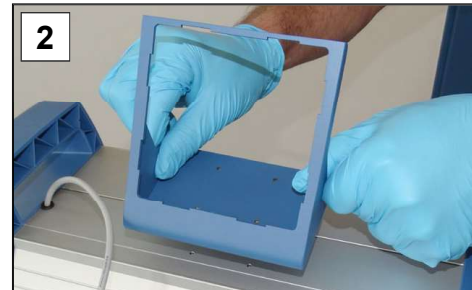
2. Position the base on the diaphragm pump.
